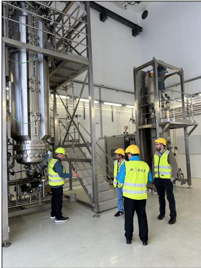
150L and 1m 3 gas bioreactors at NORCE, Risavika
