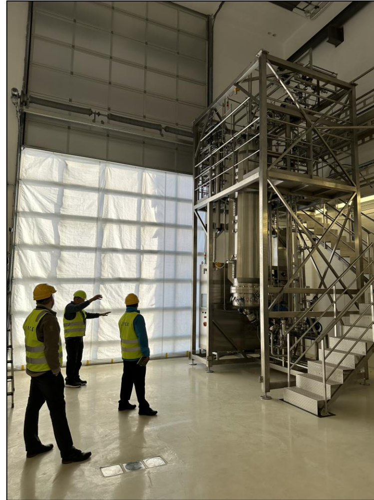
150L and 1m 3 gas bioreactors at NORCE, Risavika
