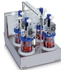
Bioreactor cultivations (1-L scale): Fed-batch at a preprogrammed growth rate of 0.03 h -1 at pH 5
