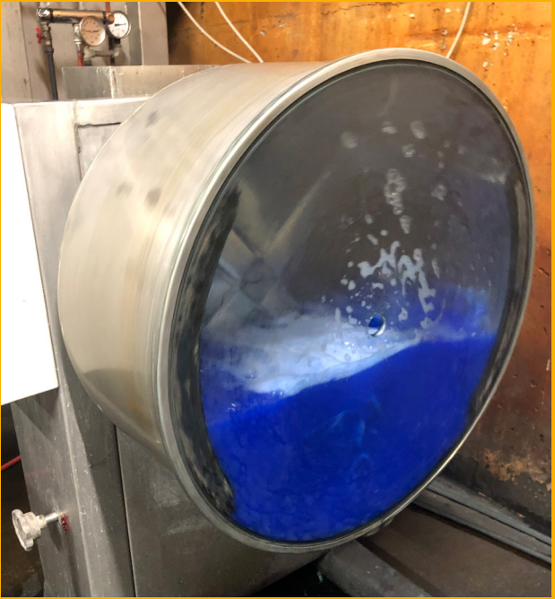
Dyeing of fish leather after tanning with sustainable formic acid. Source: Nordic Fish Leather
